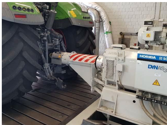
Figure 5: Dynamometer for Power-Take-Off (PTO) measurements
