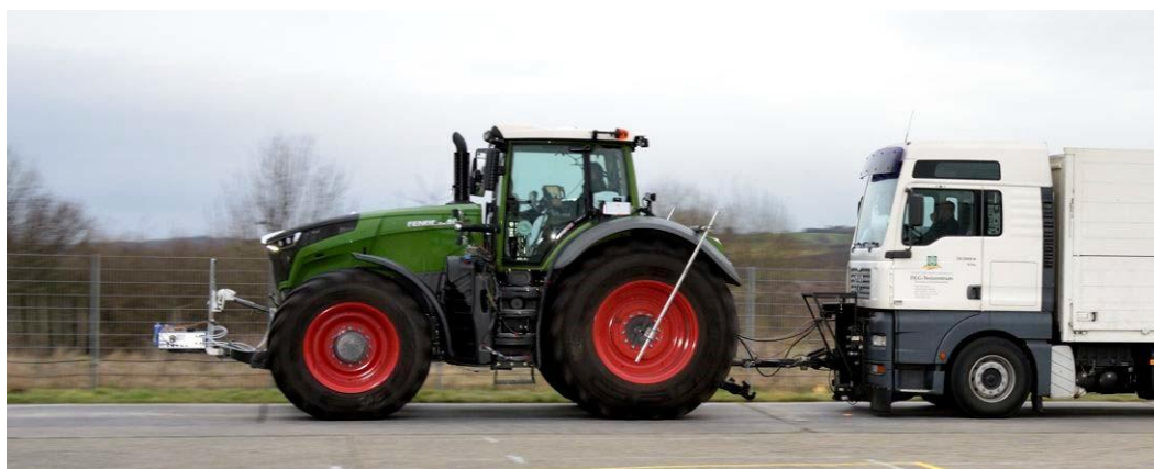
Figure 7: Specific loading vehicle for the compulsory drawbar test
