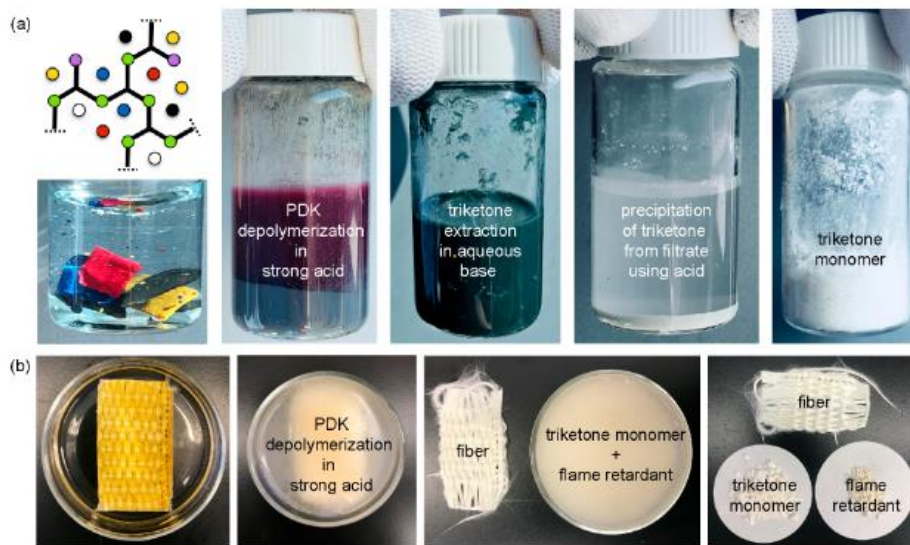
Figure 4a. Depolymerization of PDK particulates loaded with different pigments in strong acid Figure 4b. Deconstruction of a fiber-reinforced PDK composite loaded with flame retardant [Source: Christensen et al, 2019]
