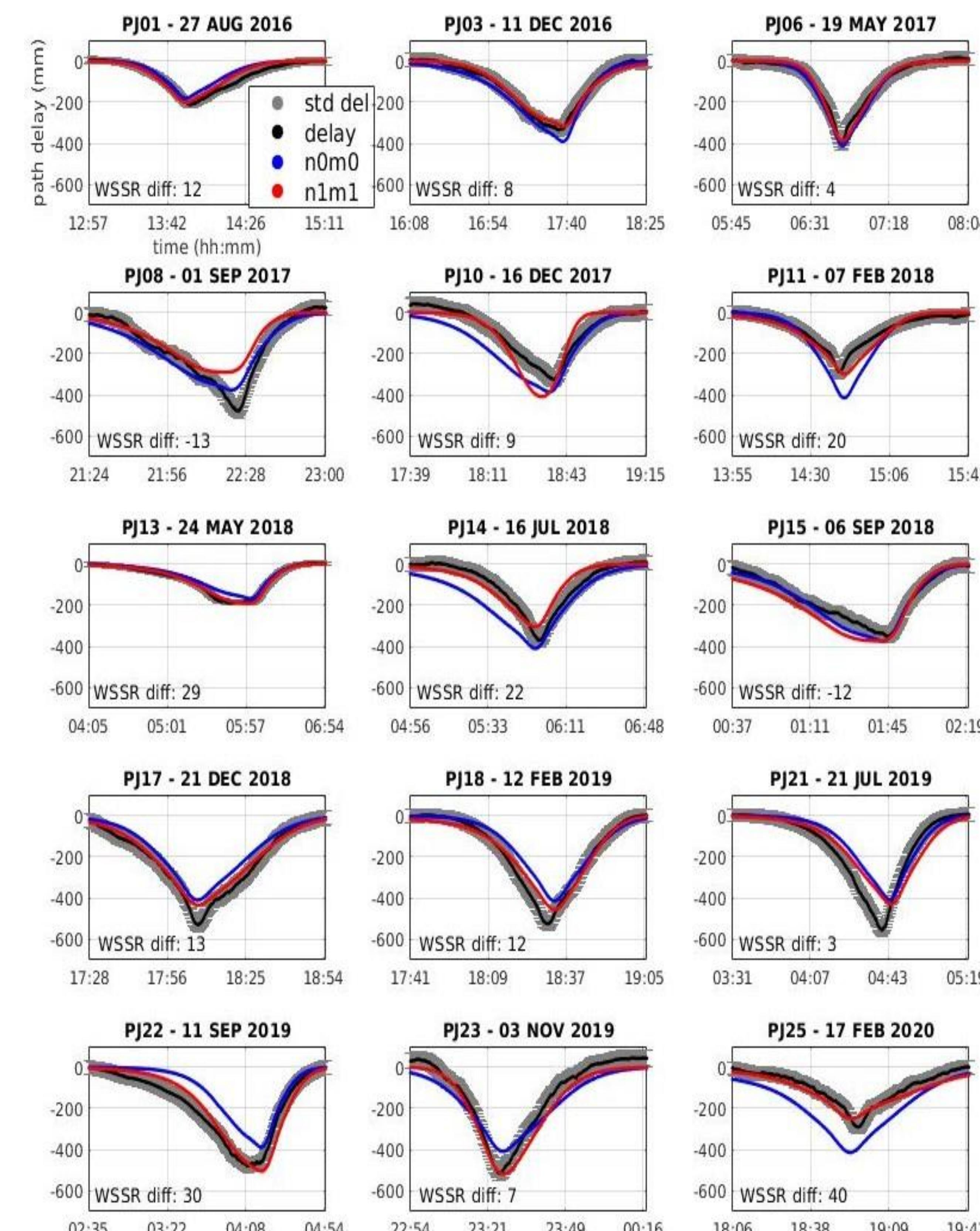
Figure 3: Fit to the path delay signature. Black: data with uncertainty (grey area). Blue: fit with an axisymmetric model (i.e: zero-order Fourier expansion). Red: fit including longitudinal and temporal variability (second-order Fourier expansion).
