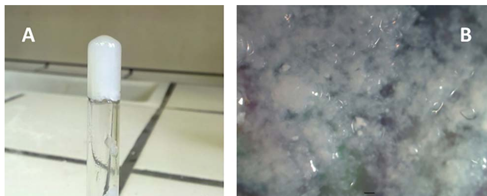
FIGURE 11 (A) Photograph of a gel obtained with a 10 mM solution of BnO-D-Oxd-L-Phe-OOC-(CH 2 ) 7 -COO-L-Phe-D-Oxd-OBn 9a in a 1:1 mixture of dichloromethane and ethyl acetate; (B) OM image of the same sample. Reproduced from Ref. 32 with permission from Wiley-VCH
