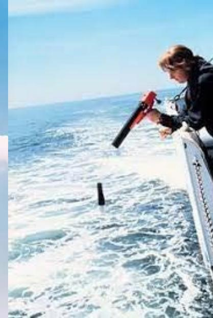
A fall-rate equations are used to derive the depth of the XBT as a function of time after the XBT is deployed into the ocean:
