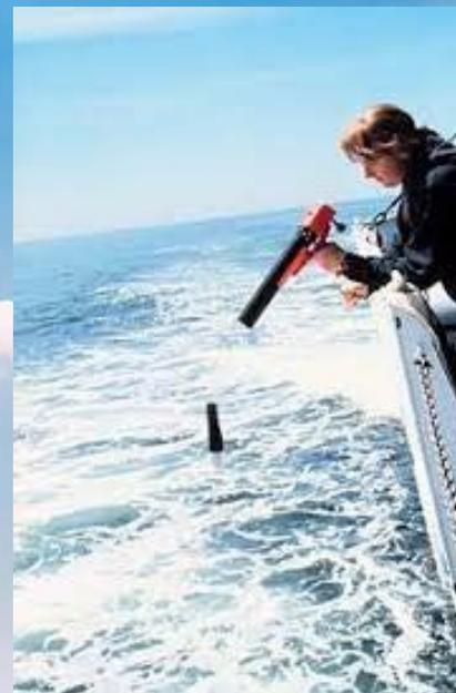
An XBT is a probe that is dropped from a ship and measures the temperature as it falls through the water
