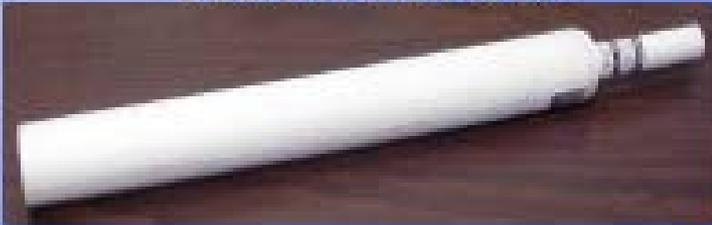
Over oceanographic temperature range, triple point of water and melting point of gallium are used as primary standards
