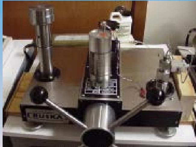
For instruments that have a strain gauge pressure sensor (Druck, Paine, Ametek, etc.), a complete pressure calibration is performed at factory, using Digiquartz pressure sensor as a secondary standard.
