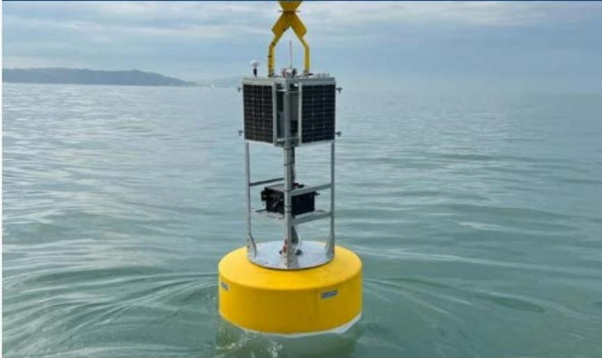
Weather-marine station installed on buoy off the coast of Fano
