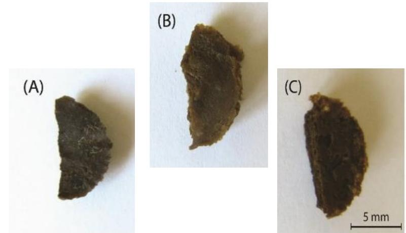
(A) the metal-treated matrix, (B) the matrix after the synthesis and (C) the EDTA-treated matrix.
