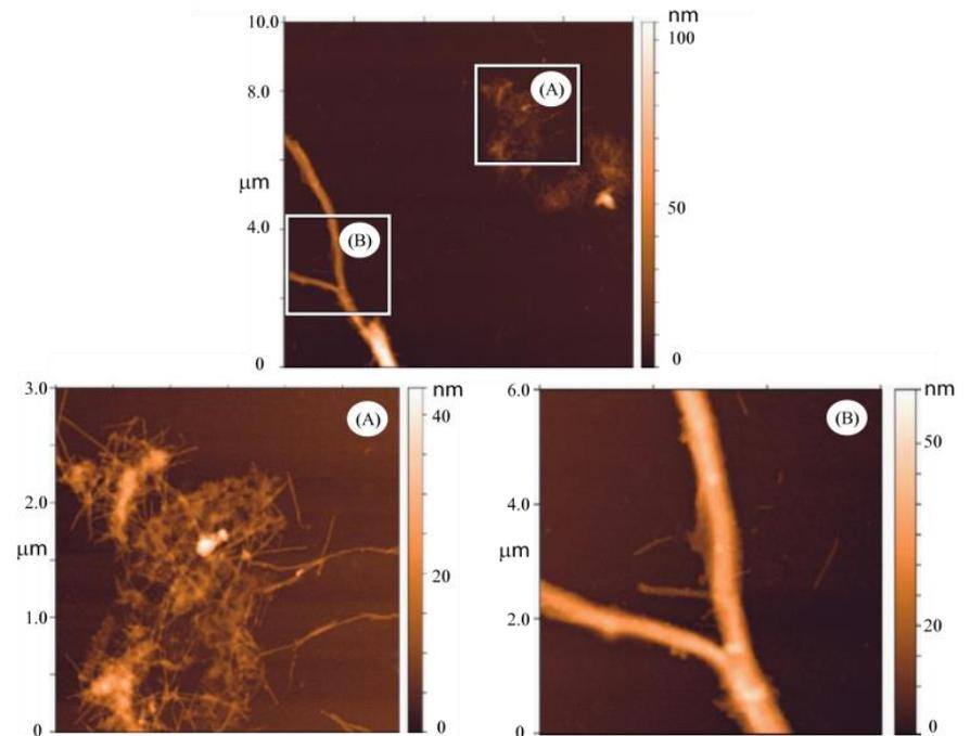
AFM images of precipitate obtained from degraded byssal threads.
