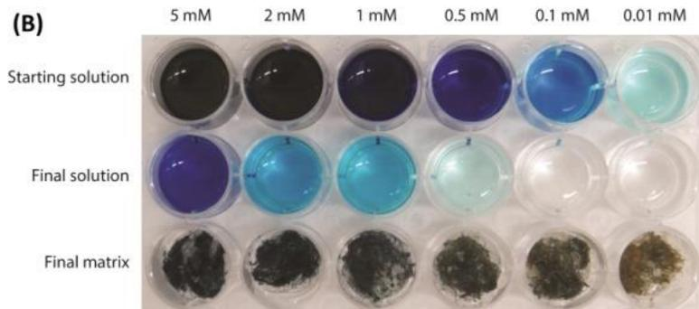
Camera photographs illustrating the dye removal experiments using (A) de-metaled byssus on EosY solutions, and (B) native byssus on MB solutions.
