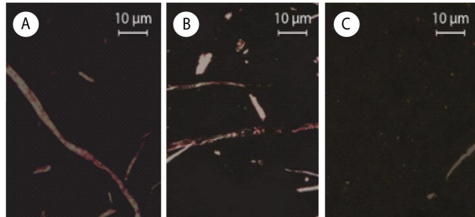
Polarized light microscopy images of the suspension obtained from the reaction at different times: 3 h (A), 6 h (B) and 18 h (C). The samples were stained with Picrosirius Red stain to enhance the birefringence of the fibers.
