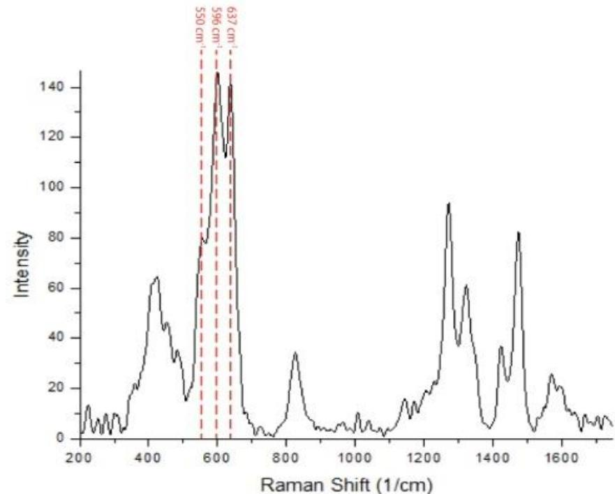
Raman spectra of a byssus matrix  $VCl_3$  treated. In red are assigned the signals of the bi-dentate chelation of the metal ion by the phenolic oxygens of DOPA.
