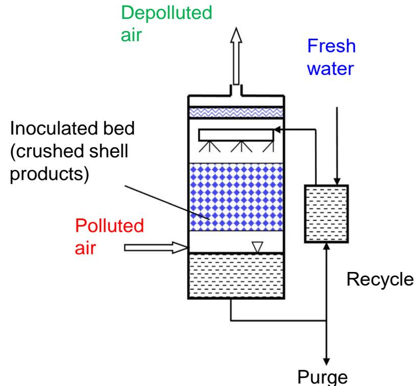
Schematics diagram of biofilter for odour removal using shell-derived materials
