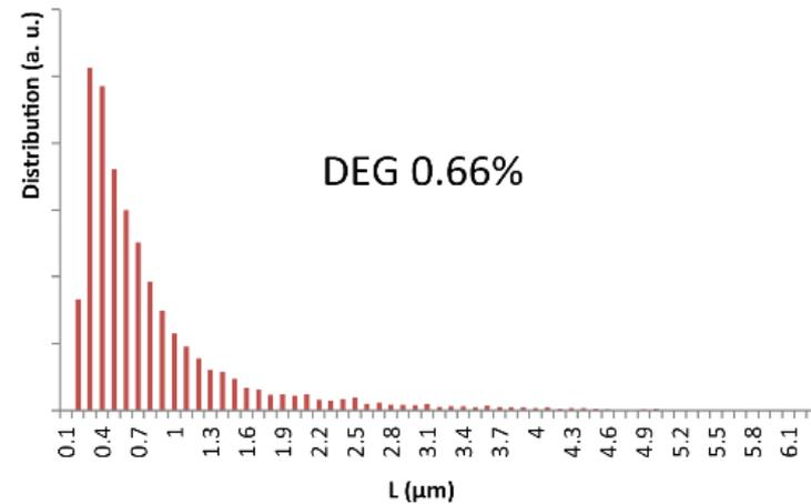
Particle size distribution of bCC after planetary ball milling grinding in the presence of different grinding aids, poly-acrylic super-fluidificant CREATIVE 4K © (CRTV) and di-ethylene glycol (DEG).
