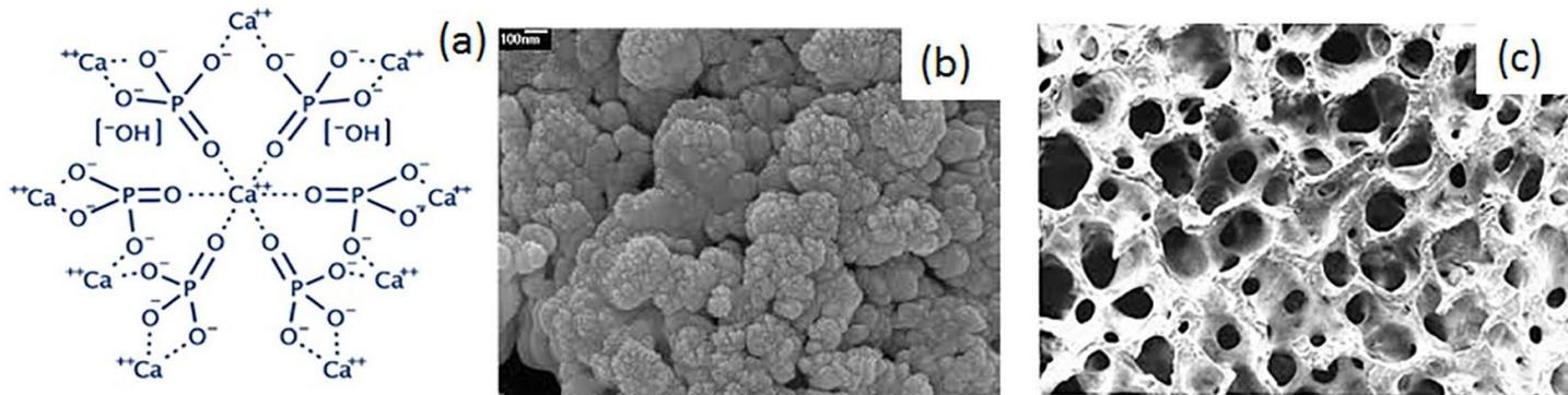
Structure of hydroxyapatite (HA) biomaterial: (a) molecular structure  $[Ca_{10}(PO_4)_6(OH)_2]$ ; (b) scanning electron microscope image of HA powder; and (c) porous microstructure of HA .
