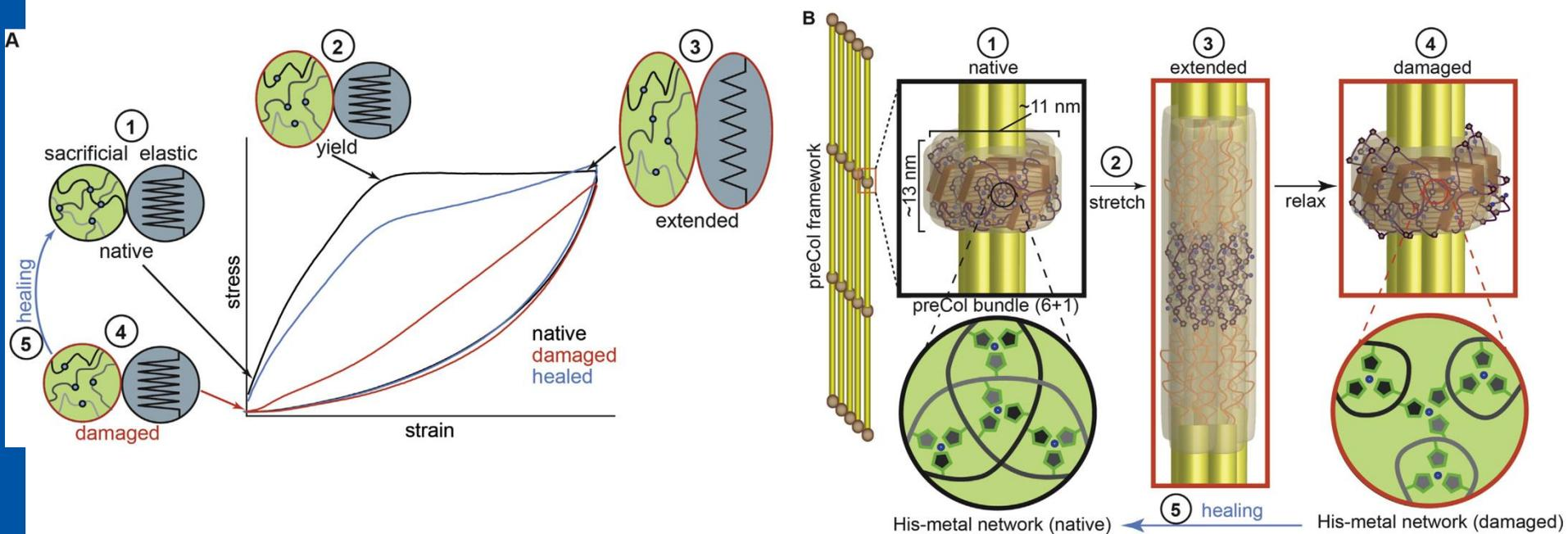
(A) Schematic illustrating changes in the preCol sacrificial network and elastic framework at specific stages of mechanical testing. (B) Schematic model at the protein level indicating changes in protein cross-linking and secondary structure at the same stages 1–5 indicated in part (A).
