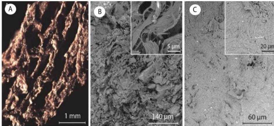
(A) Optical image of a byssus matrix transversal section. (B) SEM image of the byssus matrix section. (C) SEM image top view.
