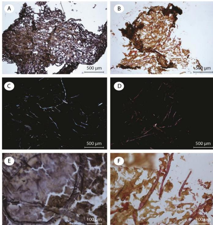
Matrix sections stained with NBT (on the left) and Sirius (on the right). A and B stained sections of the matrix. C and D are the same image observed using polarized light, to enhance the birefringent fibers. E and F are higher magnification on the fibers
