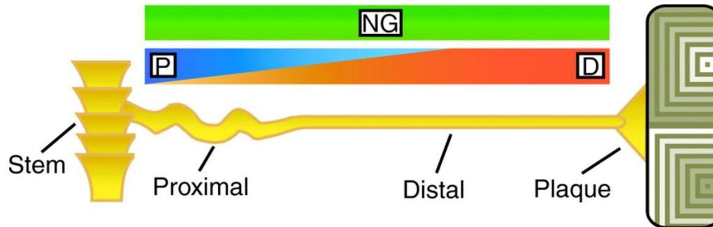
Schematic of an isolated byssal thread showing a gradient in the relative composition of preCol variants D, NG and P.
