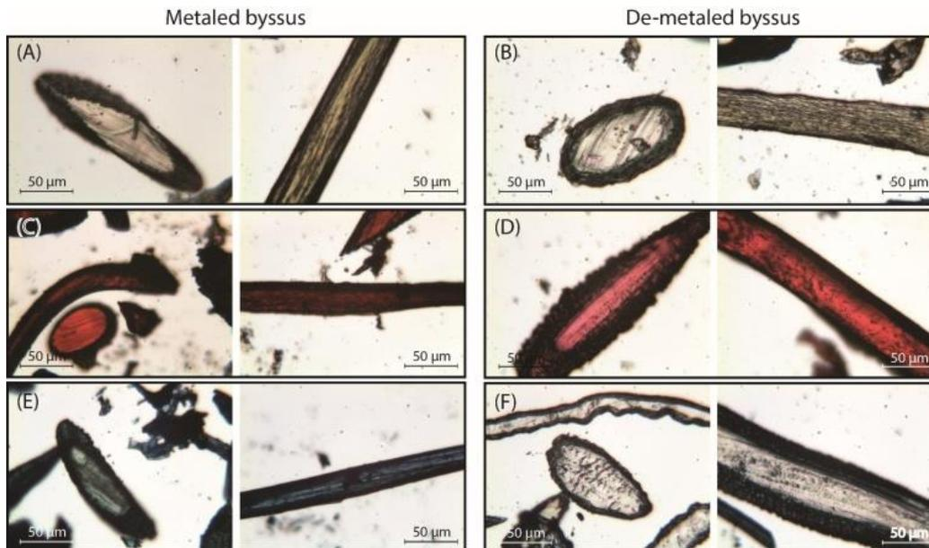
Optical microscopy images of byssus thread section of 40 mm.
