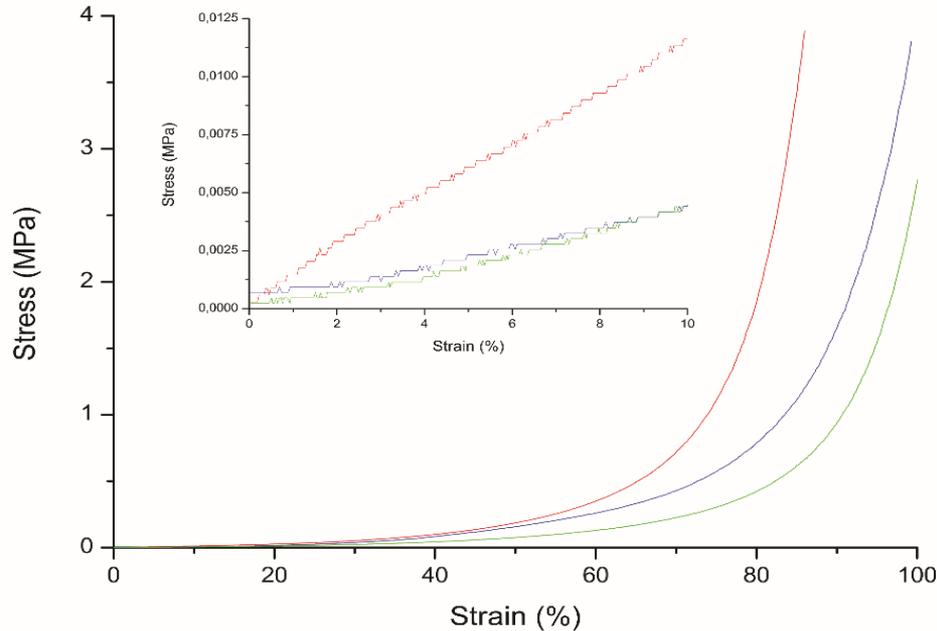
Uniaxial compression tests on the three different matrices: in red the metal-treated matrix, in green the native matrix and in blue the EDTA-treated matrix. Inset: A zoom in the 0-10% strain region.
