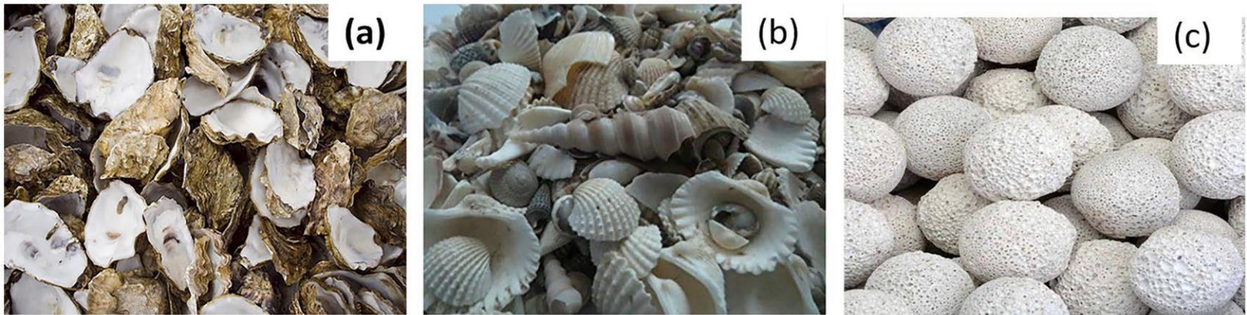
Typical biofilter media from waste shells for wastewater treatment: (a) oyster shells; (b) mixed waste shells biomaterials; and (c) shaped waste shell powder
