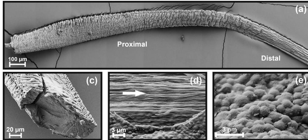
SEM images of mussel byssus of *Mytilus galloprovincialis*. (a) transition from proximal portion to the distal one; (c) cross section; (d) thread core; (e) surface structure of the byssal thread exhibiting a granular morphology;
