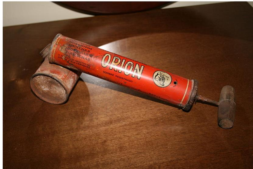
Old piston pump for DDT Used in the 60s
