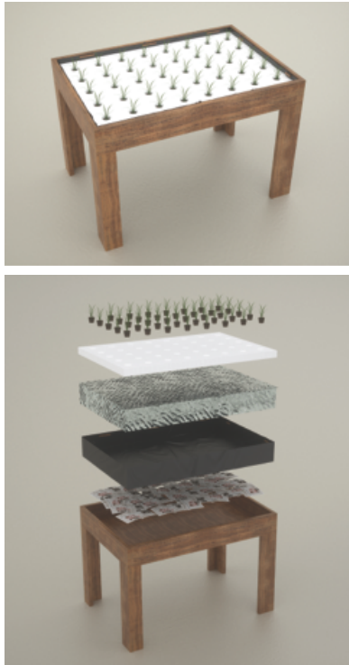
Figure 10. Basic structure of a floating system.
