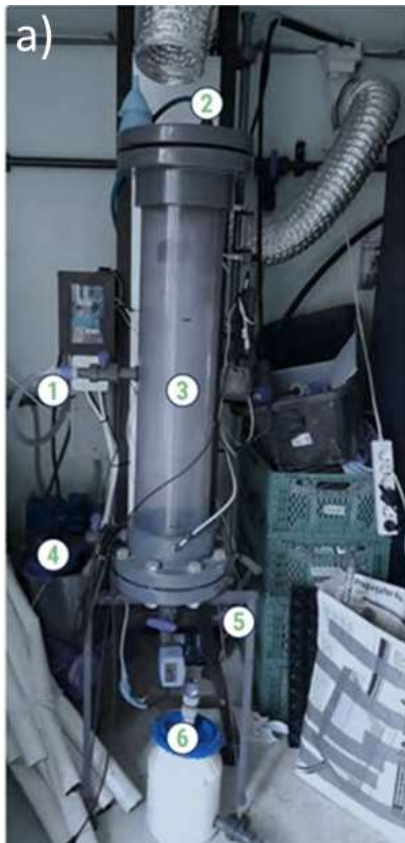
Figure 35. Semi-automated struvite reactor before (left) and after (center) connected to the sewers system, below the farm (right).
