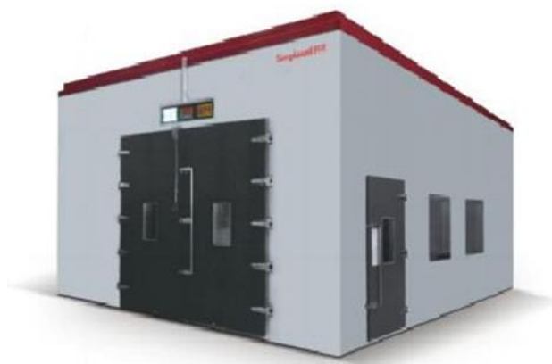
Figure 22. Isothermal chamber (Measures 830 x 566 x 290 h, Steel covered sandwich panels containing an expanded polyurethane foam inside, Sliding isothermal door (130 cm x 220 cm h).
