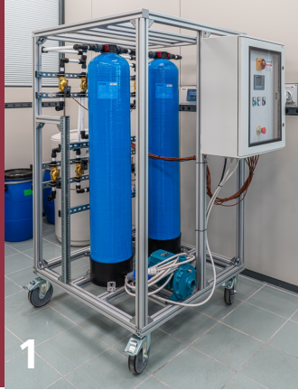
1. Pilot plant unit to test adsorption and pollutants removal
