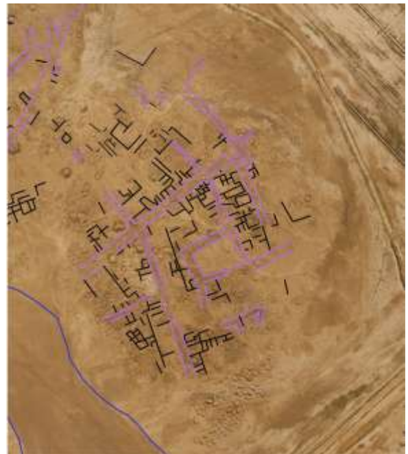
Example of identification of architectural traces on the surface of an ancient site surveyed with drones. Black lines denote possible walls, violet lines denote possible streets and alleyways.
