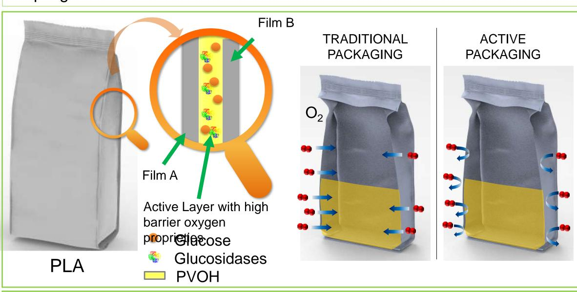
The oxygen scavenging activity is obtained by including in the multilayer film system a layer of glucose and glucosidases that catalyzes the oxygen absorption. Both the molecule and the enzyme are dissolved in a PVOH matrix and deposited on a PLA film, previously subjected to an appropriate plasma treatment in order to increase the film hydrophilicity.
