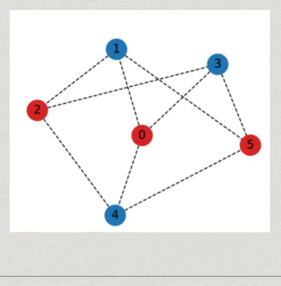
Max-Cut problem: partition the graph in two sets of nodes interconnected by the largest number of links
