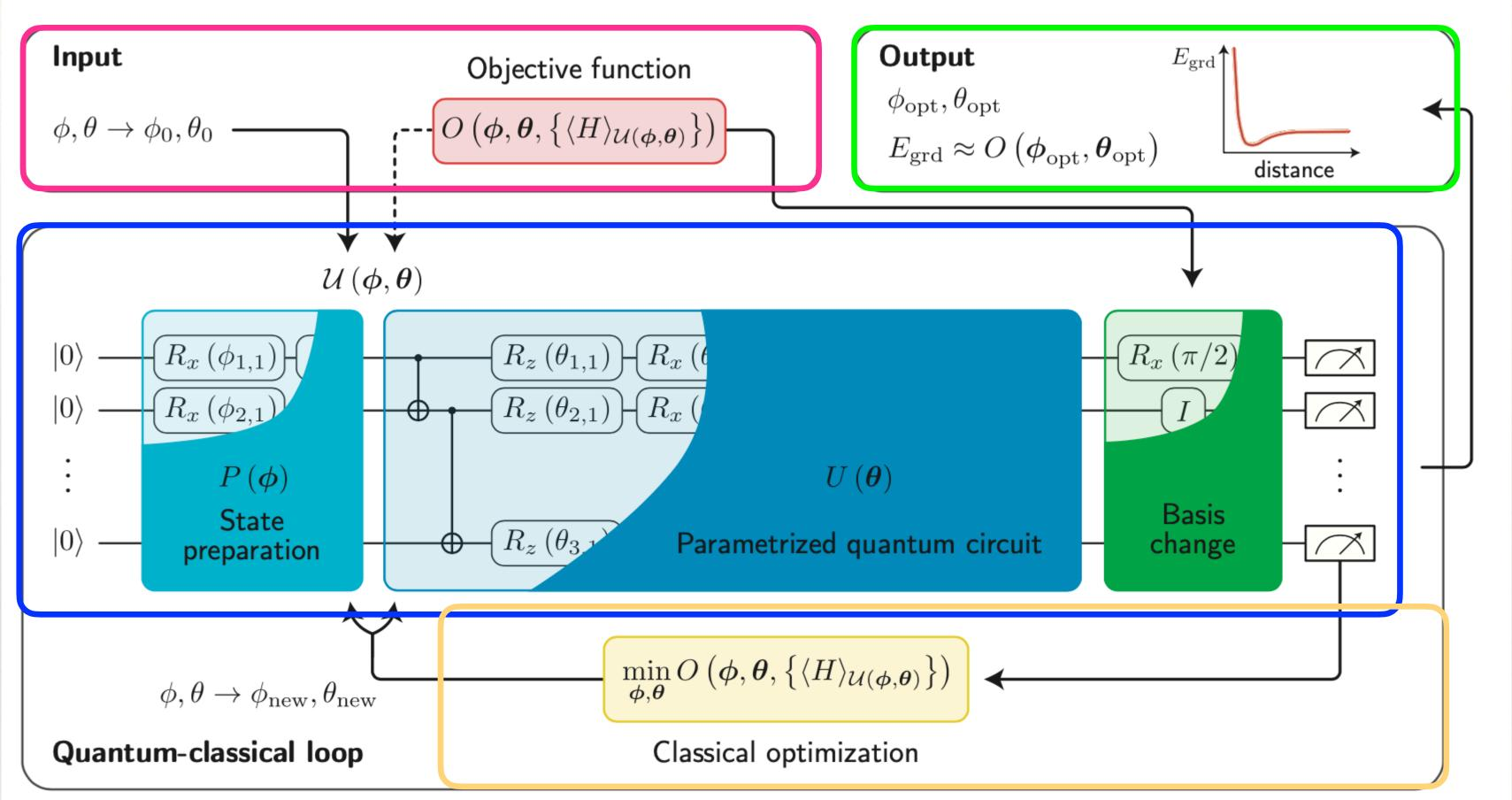
hybrid protocol: that exploits quantum resources to span the space of states and classical techniques for optimization
