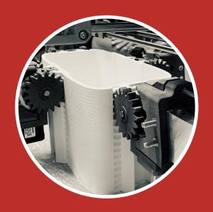
The technology consists of a 3D mobile printing robotic device able to move on the element to be printed through an integrated gripping system.
